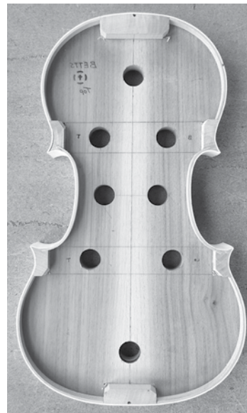
A violin mold made by John Waddle. This is what an Andrea Amati mold would have looked like.
