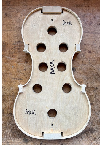
Here is a mould with the rib structure finished and ready to be removed.
