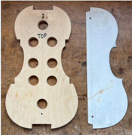
The mould and template. The template is used to shape the blocks after they are glued to the mould.
